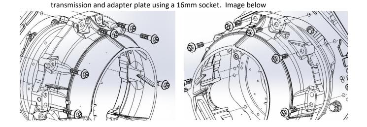
Install the (5) M12x1.75 x 50mm Flanged Hex Head Bolts in the upper holes of the
