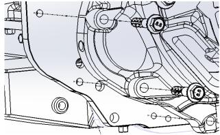
Install the (2) M8x1.25 Hex Head Bolts through the bottom two holes of the transmission into the adapter plate using a 13mm socket.
