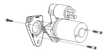
5. Bolt the Starter and Starter Block to the Adapter Plate using a 5/16'' hex key and the (2)  $3/8''-16 \times \frac{3}{4}''$  bolts.
