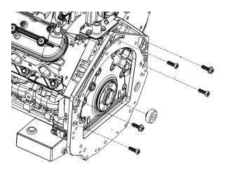
3. Press the Pilot Bearing Adapter into the LS Engine Block. Start slow and make sure the Adapter is going in square before driving it in flush.
