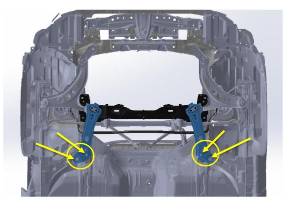
(2) Spacers go in between the front sway bar mount brackets and the unibody of the chassis on each side
