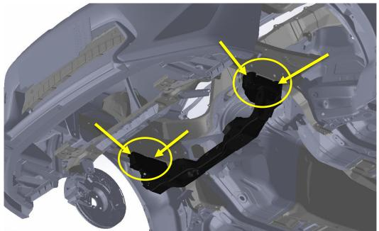
(2) Spacers go in between the front subframe and the unibody of the chassis on each side
