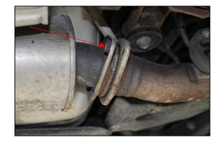
13) Remove remaining front bolts of the center X-pipe.
