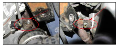
24) Unplug primary O2 (AFR) sensors. It is possible to remove the headers without taking these sensors out however you will need to transfer the sensors to the new headers or use new sensors. It is much easier to remove heat shields if sensors are removed first.
