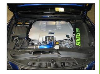
2) Remove air box cover and unplug mass air sensor from cover. Now you will be able to remove the air box. Disconnect MAF connector & harness clip located on the air-box. Remove clamp from intake tube to air-box. Remove air-box cover & filter.
