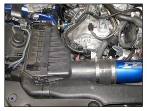
3) Disconnect VAC hose from filter housing.
