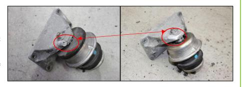
30) Reinstall mount on bracket, then reinstall engine mount assembly to engine
