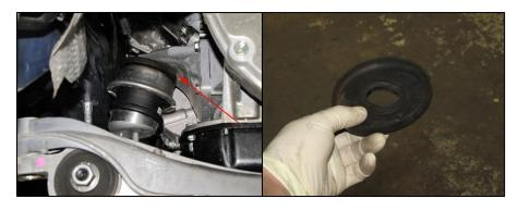
29) Remove passenger side engine mount and bracket
