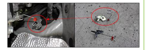
27) Remove eight nuts from each manifold. Remove stock exhaust manifolds. You may need to slightly move engine side to side and pull down on sub frame to ease removal do not raise or lower engine or damage to vehicle may occur.
