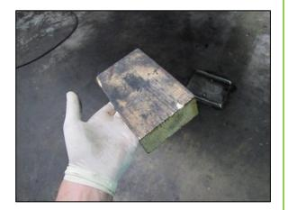
18) Place the block of wood on top of the stand. Lift the stand until the wood is putting pressure on the crank pulley and timing cover to support the weight of the engine. Make sure wood is straight, this will support engine during header
