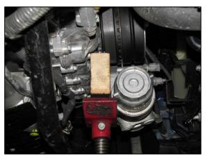
19) Remove both nuts on the bottom end of the engine mount bushings 17 mm.
