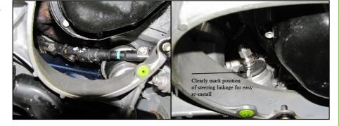
17) Remove steering shaft and remove the bolts from either end of steering U-joint. Ensure that the marks are clear. You may want to extend the marks when disassembled to allow for the reassembly process to be uncomplicated while also retaining proper alignment. *Note which side of the joint is the top for they are not alike.*
