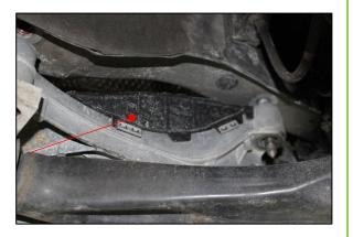
23) Remove dampers from motor mounts on both sides secured by a single 10mm bolt. (will be reused)
