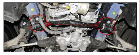
16) Clearly mark the steering shaft and steering shaft joint connection points as well as the connection point between the joint and steering rack.
