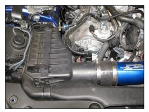
3) Disconnect VAC hose from filter housing.
