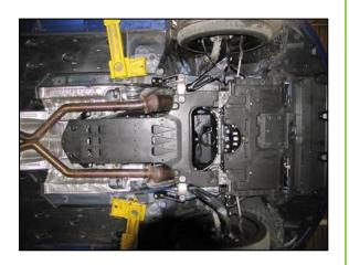
8) Remove both sway bar splash guards – both sides are secured with a singular bolt and clip. *Take care to avoid breaking when removing said clips*.
