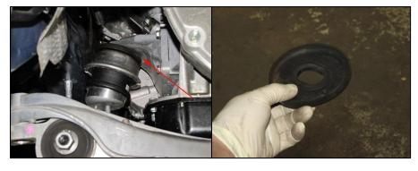
29) Remove passenger side engine mount and bracket Separate engine mount and bracket Remove rubber from engine mount Cut / grind the displayed bolt hole on the engine mount bracket until
