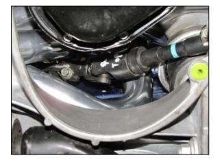
38) Install X-Pipe and brace from trans to header flanges, using original hardware and with supplied header to X-pipe gaskets.
