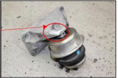
30) Reinstall mount on bracket, then reinstall engine mount assembly to engine
