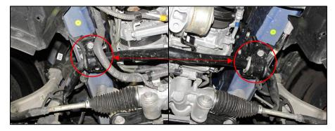
steering shaft joint connection points as well as the connection point between the joint and steering rack. This step will ensure your alignment when reassembling the vehicle. Although we do
