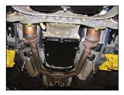
10) Remove converter support Bracket from exhaust & transmission.
