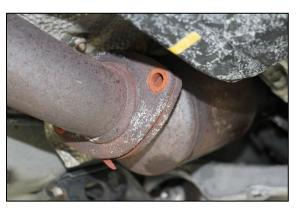
14) Remove center section of exhaust X-Pipe.
