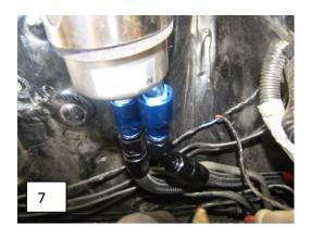
Step 5- Now tighten the fittings to the fuel filter. Do not over tighten AN fittings, they can be damaged very easily.
