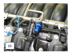
Step 8- Install the 90degree fuel feed hose fitting onto the rail fitting. Route hoses towards the back of the intake manifold.
