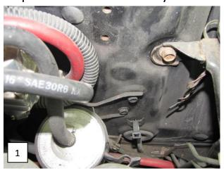
Step 2- Take supplied fuel filter with the original fuel filter bolts and reinstall. Use the upper hole location, not the same holes where the factory one was installed (Fig 2 &3).
