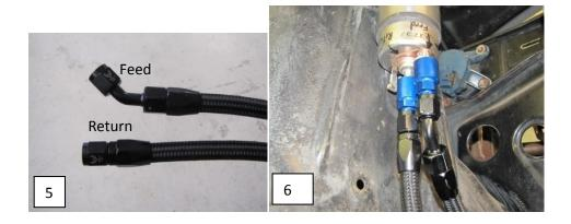
Step 4- Clamp the supplied lines onto the existing factory lines.
