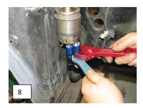
Step 6- Install the fuel rail feed hose to the fuel filter.
