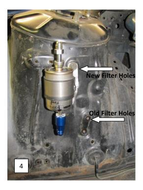
The center line on the fuel filter is the return and the outer line is the feed.
