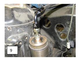
Step 7- Install the supplied clip on fitting onto the fuel rail.
