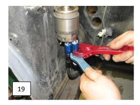
Step 11- Install the fuel rail feed hose to the fuel filter.
