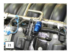
Step 13- Install the 90degree fuel feed hose fitting onto the rail fitting. Route hoses towards the back of the intake manifold.
