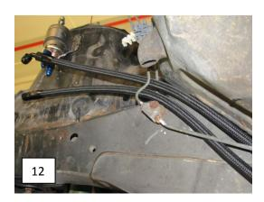
Step 6- Loosely start the fittings onto the fuel filter.
