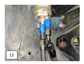
Step 7- Zip tie lines, at the front, to the factory hard lines as needed to remove slack.
