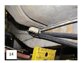
Step 8- Take the cable clamps and install. Mount the first clamps on in a location in front of the oval tow hook. Mount the second ones just past the break in the frame rail seam. Bend the clamp tabs up for clearance.
