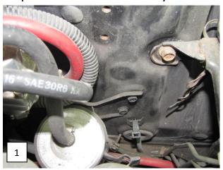
Step 2- Remove fuel hoses and lines back to the fuel tank. To gain access to the fuel pump go through the trunk. Remove the push pins and pull up the carpet.
