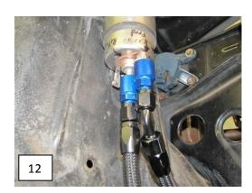
Step 7- Zip tie lines, at the front, to the factory hard lines as needed to remove slack.
