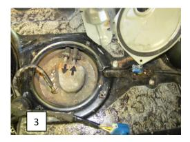
Step 3- Take supplied fuel filter with the original fuel filter bolts and reinstall. Use the upper hole location, not the same holes where the factory one was installed (Fig 6 &7).
