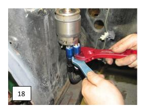
Step 11- Install the fuel rail feed hose to the fuel filter.
