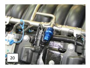
Step 13- Install the 90degree fuel feed hose fitting onto the rail fitting. Route hoses towards the back of the intake manifold.
