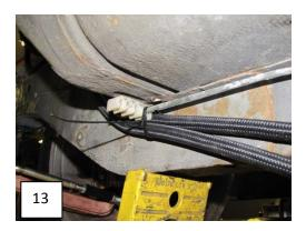
Step 8- Take the cable clamps and install. Mount the first clamps on in a location in front of the oval tow hook. Mount the second ones just past the break in the frame rail seam. Bend the clamp tabs up for clearance.
