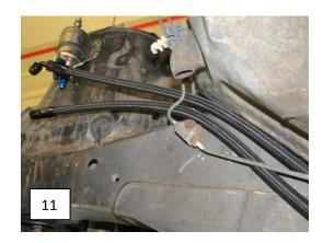
Step 6- Loosely start the fittings onto the fuel filter.
