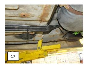
Step 10- Go to back to the front and tighten the fittings to the fuel filter. Do not over tighten AN fittings, they can be damaged very easily.
