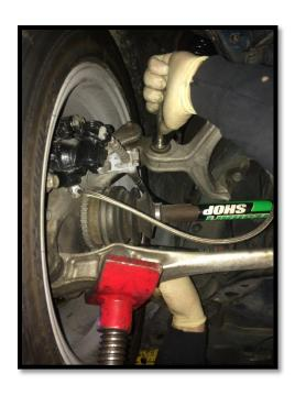
3- Now you can install the Sikky endlinks. As with the front endlinks, you can flip the large spacer on the upper heimjoint as needed to allow the endlink to reach the different hole locations.
