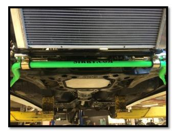
5- Install the Sikky endlinks. You can move the big spacer on the upper heimjoint as needed to allow the endlink to reach the different hole locations. Our slotted sway bar bushing brackets also allow you to slide the bar as needed.
