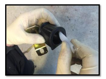
4- Install the bushings and brackets onto the outer edge of the sway bar. Then install the bar onto the relocation brackets.
