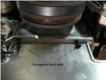
Install the rest of the stock bolts into pan, but only finger tight.
