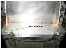
Install the two lower bell housing black bolts to position the oil pan correctly, *Tighten until pan is flush with engine block. Do not set until final torque.*
