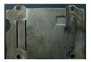
Reinstall factory baffle, leaving off front left windage tray bolt.
