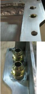
Apply sealant to dipstick fitting and thread into bung on top of oil pan \**do not over torque*\*
