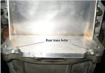
Tighten the rest of the stock bolts into engine blocks to 25 Nm (18 ft. lbs.). Tighten the bell housing bolts.
