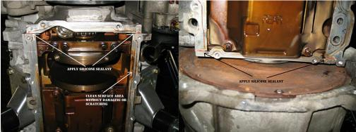
Using bolts holding gasket to oil pan, start to fit oil pan to engine block; get bolts started but do not tighten.
