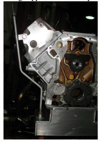
When installing the oil filter relocation kit be careful not to route the lines too close to your headers. The heat can damage the coating on the inside causing them to leak. And also be sure to install the lines correctly. OUT on the oil pan goes to IN on the filter block, OUT on filter block goes to IN on the oil pan. This creates a full cycle and if reversed you will not have oil pressure.
