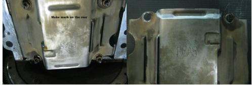
Cut marked area, grind all excess metal until all metal shavings are clean.
