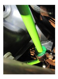
Step 12. Once the bushings are properly aligned, you can now tighten the four 12mm bushing retainer bolts.
