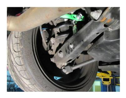
Step 18. Fully tighten down the endlink nut. The endlink bolt is 16mm and the nut is 19mm.
