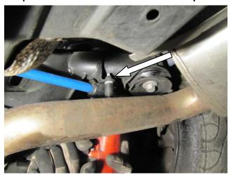
Step 5. Pull the factory endlinks up and out of the control arm. Rotate the bar and slide out towards the driver side.
