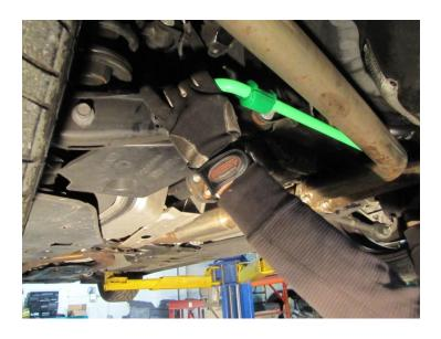
Step 10. Reinstall 12mm sway bar retainer bolts- do not tighten.
