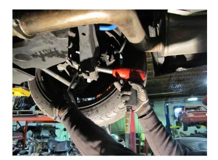
Step 3. Remove the lower sway bar 12mm link nuts.
