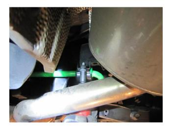
Step 13. Rotate the bar out of the way to make clearance for the sway bar endlinks. Slide bottom of endlinks into place and align with hole.
