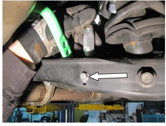
\*NOTE: On the driver's side make sure the ride level sensor is attached like the factory setup.
