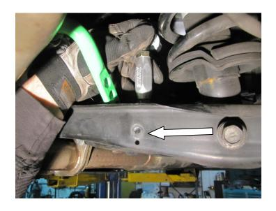
Step 14. Start the 12mm sway bar retainer bolts. Do not tighten.
