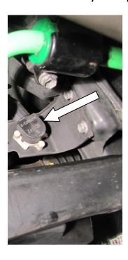
Step 15. Install the upper sway bar link into the hole of your choice. The correct order is- washer, sway bar, washer, and nut. Now hand tighten the nut. Do not tighten the jam nuts located above and below the endlink turn buckle, leaving free play adjustment.
