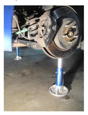
Step 3: Lower vehicle till all weight is supported by the jack stands. The suspension now has full load on it.
