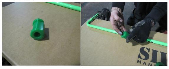
Step 7. Open the bushing where it is sliced and slide over the sway bar. Position as shown.
