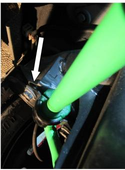
Step 11. After all bolts have been started make sure the bushing is properly installed. It needs to be aligned and centered as shown.
