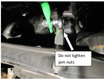
Step 16. Once the endlinks are in tighten the lower 12mm sway bar retainer bolts.
