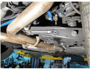
Step 4. Remove the 12mm sway bar retainer bolts.
