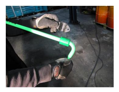
Step 9. Slide bar into place from the driver side to the passenger side.
