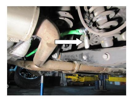
Step 5. Now that the turn buckle is free, twist is clockwise until it stops and note the position. Then twist it counter clockwise until it stops and note the position. Center the turn buckle in between the 2 noted positions and you will be set at zero pre load.
