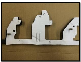
3- Using a ¼" drill bit, drill the holes out accordingly.
