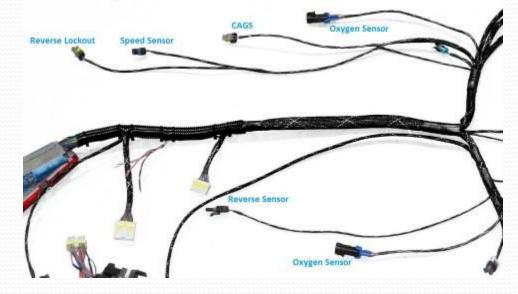
To avoid improper installation on the transmission sensors, a diagram has been provided. Again, note that laying out the harness in the early stages is crucial for proper fitment.
