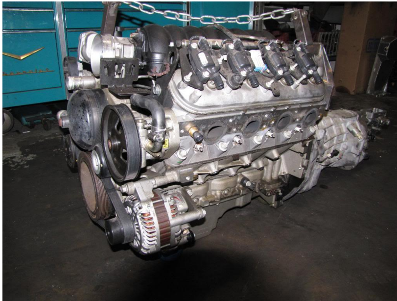
Donor LS2 engine and 6 speed manual trans from a 2006 Pontiac GTO
