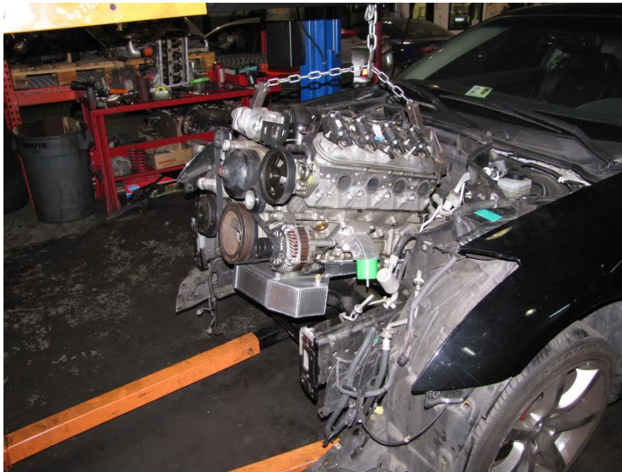
Begin install of new engine and trans. Install is as easy as bolting up the VQ with our kit.
