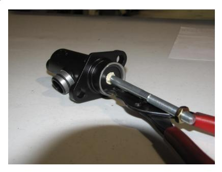
4.) Re-assemble the Wilwood master cylinder using the stock Nissan push rod, with the Sikky provided washer, and the Wilwood snap ring.
