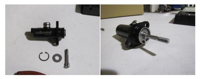
5.) Thread on the Sikky provided jam nut, Sikky push rod adapter, another jam nut, and the Nissan U-Bracket, in that order, to end of the Nissan push rod.
