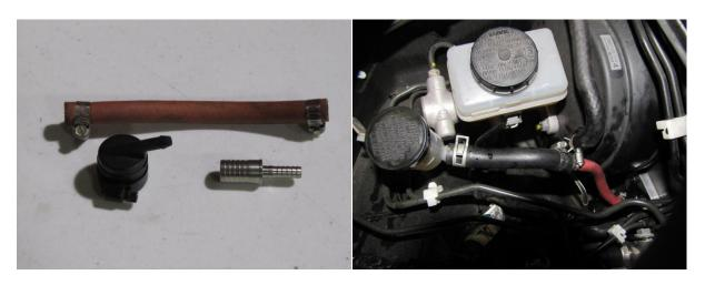
9.) Install the master cylinder to the firewall by lining up the bolts on the Sikky Adapter plate to the stock master cylinder bolt holes on the firewall. Fasten into place by threading the 2 provided lock nuts on to the bolts from inside the car, and final tighten into place.
