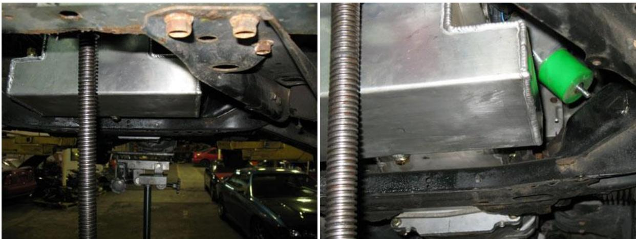
Once out of the bolt hole locations, carefully push engine toward the passenger side engine bay. This extra clearance will allow you to install the **driver side header FIRST!**
