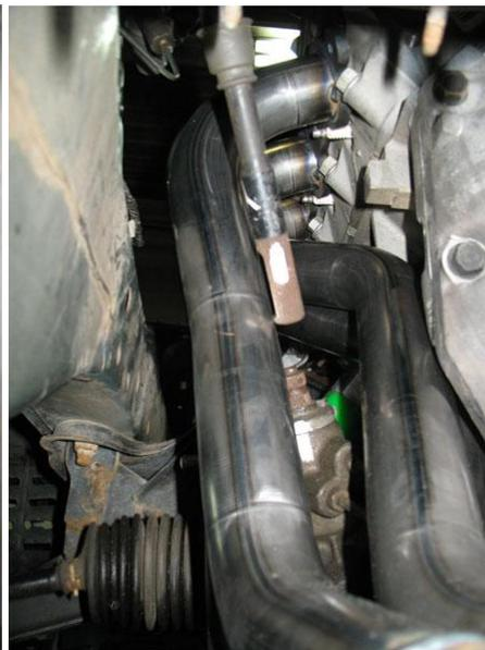
When you have the steering column rod in place, install a bolt in the front bolt hole of the header flange. Then bolt the rear header bolt in, but do not tighten all the way, leave loose, about 1/8<sup>th</sup> inch gap between header so you can slide gasket into place later.
