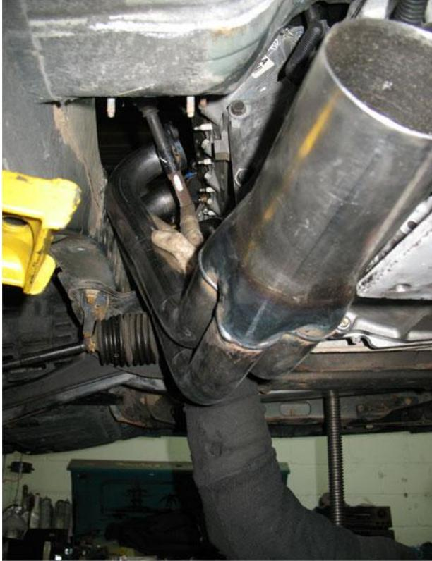
Cut zip tie that is holding steering column rod and begin to work it through the header
