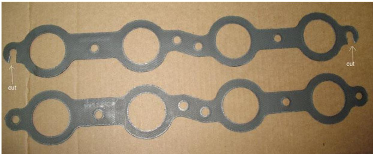
Now you can drop in gasket through 1/8<sup>th</sup> in gap and begin inserting supplied hardware to tighten down both passenger side and driver side headers.
