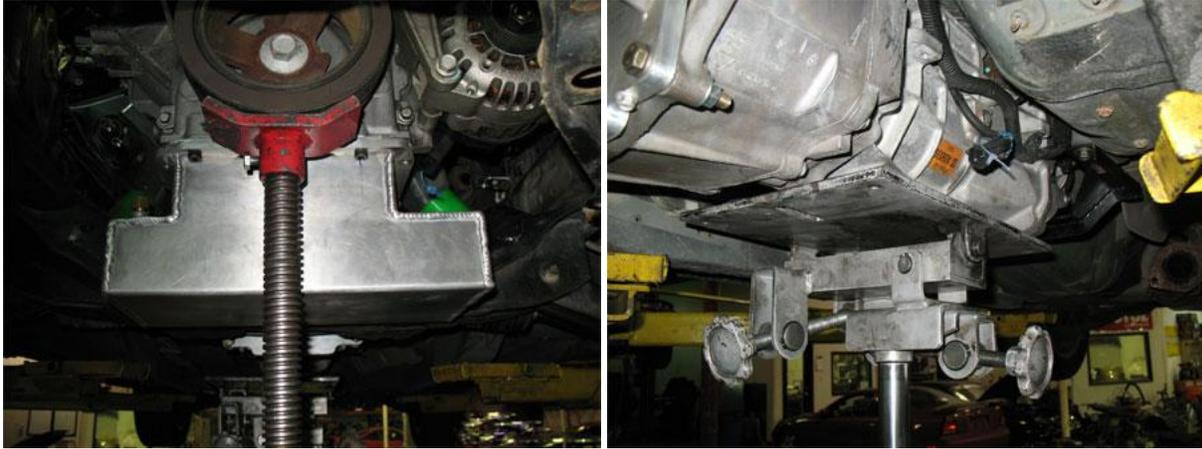
Next unbolt the transmission bracket and begin to lower down until at a 15 degree angle to the back of the car and begin lifting the front of the motor by the crank pulley until the motor mounts barely come out of the stock bolt hole locations.
