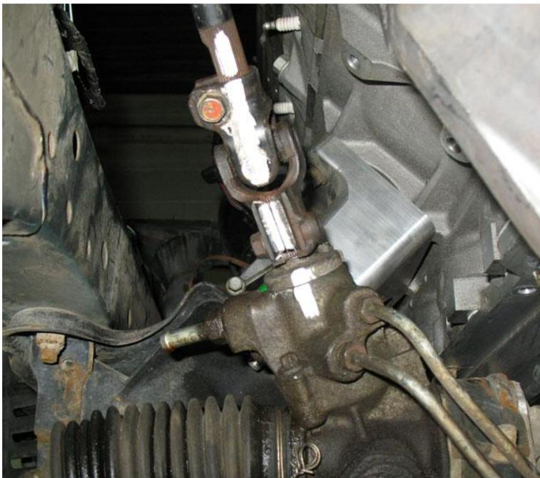
Completely remove steering universal joint, make sure you note bottom from top.
