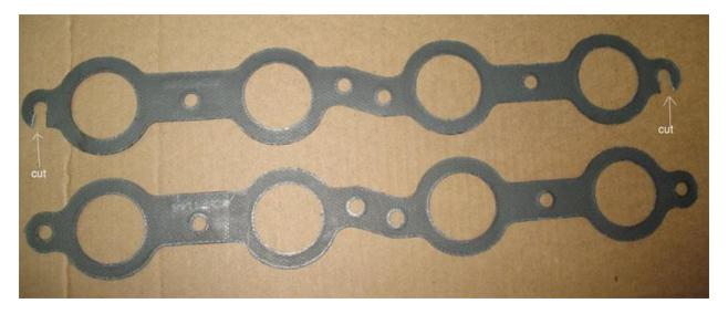
Now you can drop in gasket through  $1/8^{th}$  in gap and begin inserting supplied hardware to tighten down both passenger side and driver side headers.
