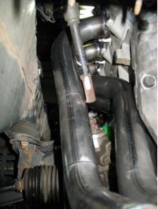
When you have the steering column rod in place, install a bolt in the front bolt hole of the header flange. Then bolt the rear header bolt in, but do not tighten all the way, leave loose, about  $1/8^{th}$  inch gap between header so you can slide gasket into place later.
