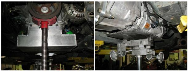
Next unbolt the transmission bracket and begin to lower down until at a 15 degree angle to the back of the car and begin lifting the front of the motor by the crank pulley until the motor mounts barely come out of the stock bolt hole locations.
