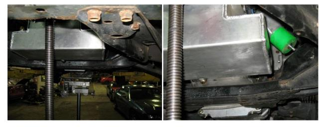
Once out of the bolt hole locations, carefully push engine toward the passenger side engine bay. This extra clearance will allow you to install the **driver side header FIRST!**
