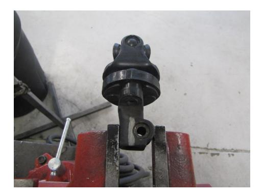
8- With a cut off wheel or grinder cut the heads off the solid rivets
