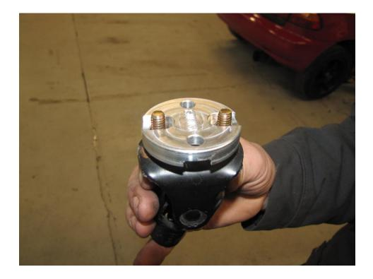
Step 18- Install the supplied nuts into the bushing slots and tighten them from the other side to making sure they are seated properly in the stopper slots.
