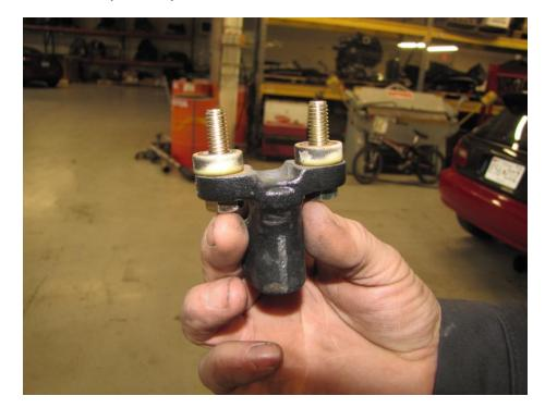
Step 20- Install the spacers you saved onto the new bolts
