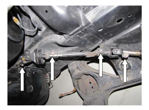
6- Slip steering linkage together and remove from the car. Make sure if you're using oil that you don't remove the marks you made
