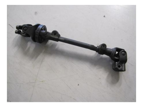
7- Remove the universal from steering linkage and place in a vice like pictured. The upper link has a rubber bushing; you'll want the cast side in.
