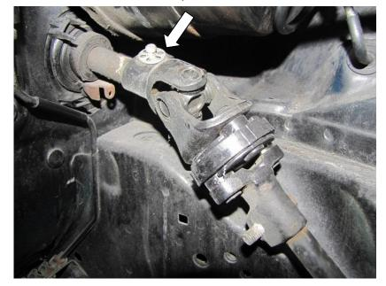
3- When this bolt is removed the clip can be discarded
