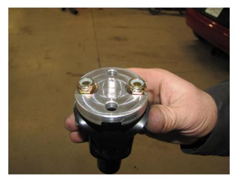
Step 19- Take the cast side of the universal and install the supplied bolts facing down like pictured
