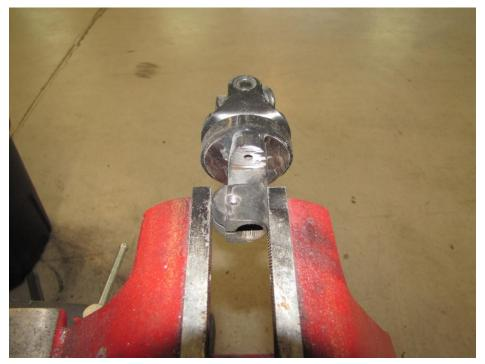
11- With a center punch you'll need to hammer out the rivets. They are tight so you may need to adjust your hammering angle to get them out.
