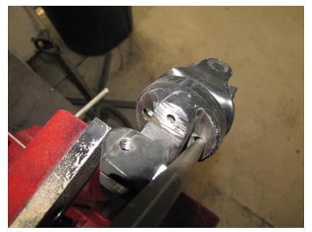
12- Completely remove rivets from both sides of the universal.
