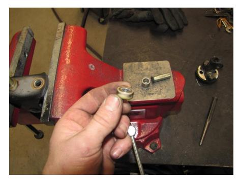
14- Remove the riveted rubber bushing, saving the plastic spacers
