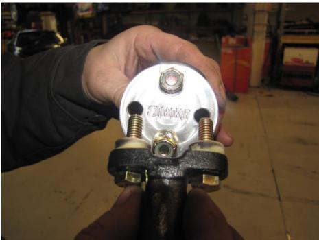
Step 22- Install the supplied nuts and tighten from the splined side of the cast piece. Make sure the nut is seated in the stop slots.
