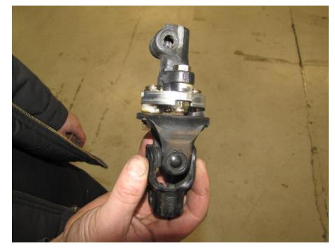
Step 23- Reinstall the steering column aligning the marks your previously made. Then tighten the bolts you saved and check steering to make sure its strait
