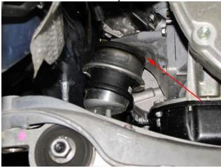
30. Pull rubber off top of mounts and reinstall
