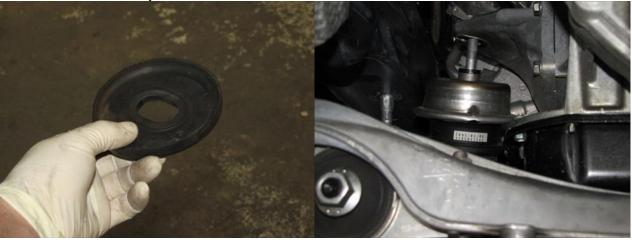
31. Recommend using 2 small pieces of tape (any kind strong enough to hold gasket) between exhaust parts on gasket to hold to head
