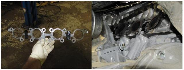
32. Install one header at a time: Lifting, lowering and shifting motor as necessary to start all bolts
