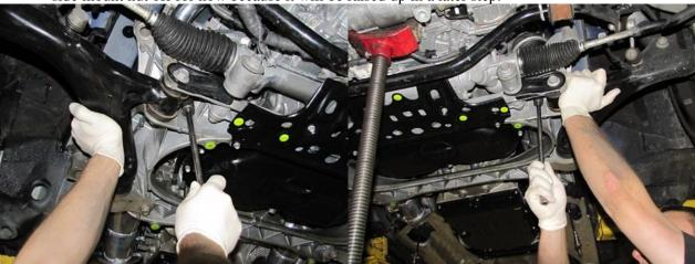
36. Next push up on control arm and carefully start front sub frame bolts (19 mm)
