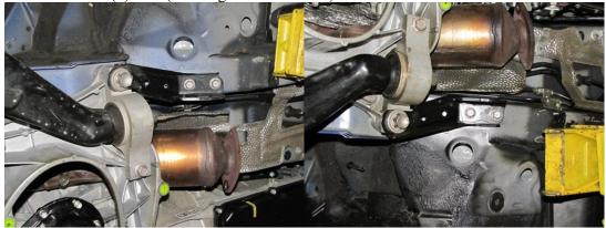
19. Remove motor mount bolts (2) 17 mm
