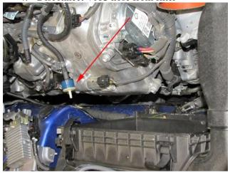
Remove 10mm bolt from passenger side valve cover that retains dipstick
