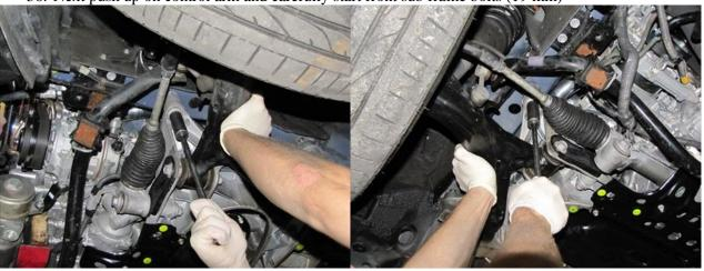
37. Now install rear control arm sub frame tow hook bracket main bolts (7/8") DO NOT TIGHTEN
