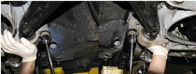
38. Now start 14 mm bolts in the tow hook brackets ( DO NOT TIGHTEN)
