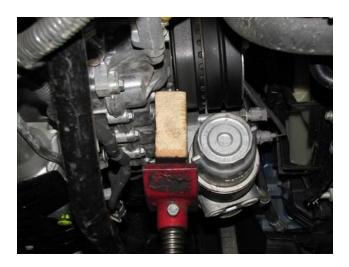
16. Clearly mark steering shaft with lines from knuckles to shafts and mark top (there is a long and short side)
