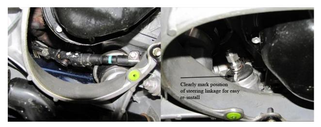
17. Remove steering shaft universal and mark solid marks (may want to extend marks for easy install)
