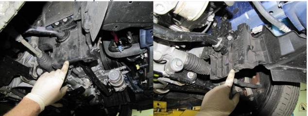
9. Remove secondary O2 sensors from exhaust pipe (you do not need to unplug) Unscrew sensors and leave them hanging
